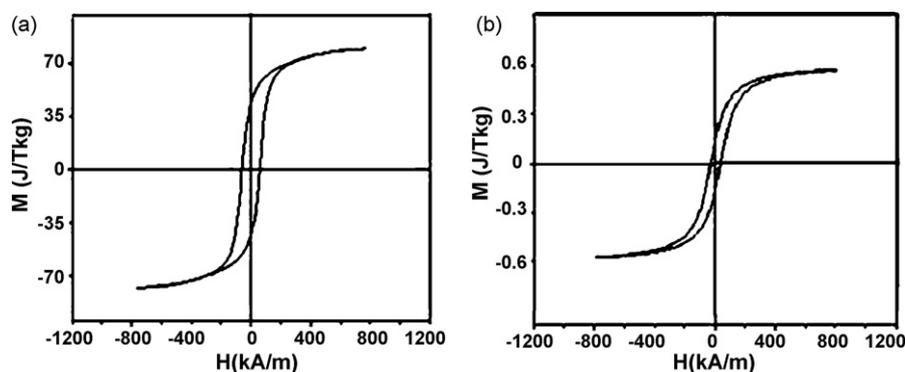
Fig. 5. Magnetization curves of (a) cobalt ferrite and (b) MCM-41/CoFe<sub>2</sub>O<sub>4</sub> nano-composite.
