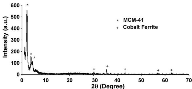
Fig. 3. XRD pattern of MCM-41/CoFe<sub>2</sub>O<sub>4</sub> nano-composite.
