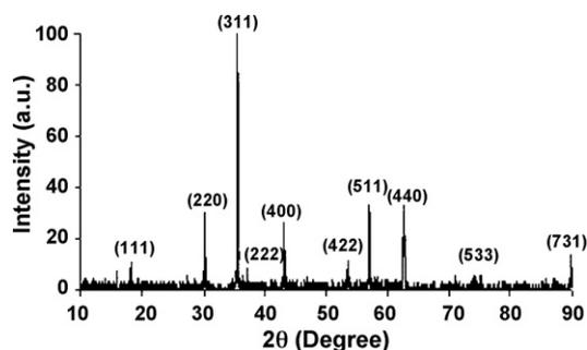
Fig. 1. XRD pattern of cobalt ferrite synthesized under the given experimental conditions.
