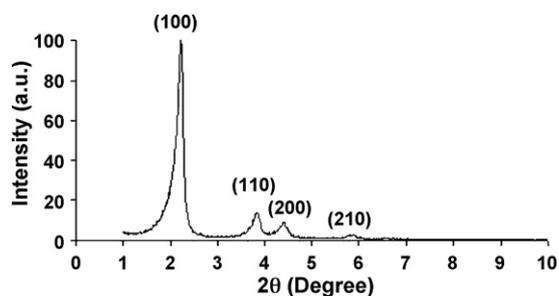
Fig. 2. Low-angle XRD pattern of processed MCM-41.
