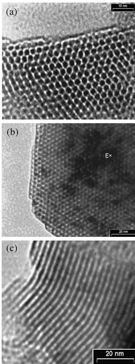
Fig. 4. TEM images of annealed MCM-41 (a), MCM-41/CoFe<sub>2</sub>O<sub>4</sub> nano-composite through the pore axis (b) and along the channels (c).
